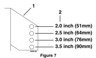
For cutting heights above 3.5 inches (38 mm) use the bottom hole. The rollers will still be effective against scalping.
